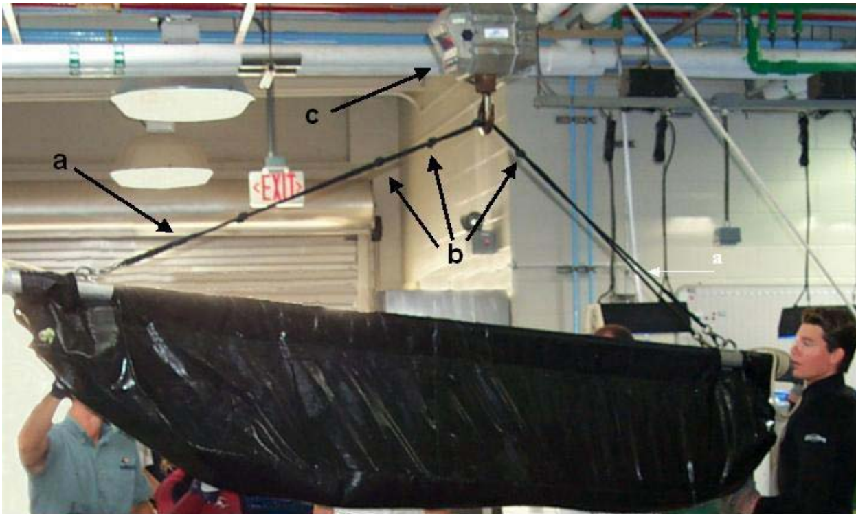
Figure 20.5. Weighing a shark using a stretcher suspended from the ceiling by a knotted rope (a), with knots approximately 20 cm apart (b), and a digital scale (c).
