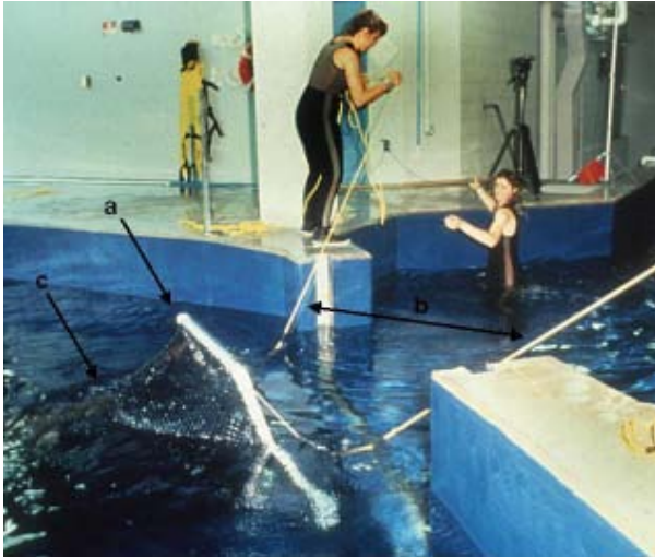
Figure 20.1. A box net used to capture sharks. The box net is constructed of a 5 cm diameter PVC pipe frame (a), two guide ropes on opposite sides of the frame (b), an additional guide rope attached to the bottom of net (not seen), and 2.5 cm x 2.5 cm mesh netting (c).
